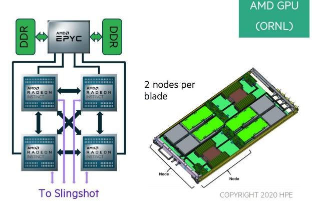
9,472 nodes, each with 1 AMD EPYC 64 core CPUs and 4 Radeon Instinct MI250X GPUs 606,208 CPU cores and 8,335,360 GPU cores
